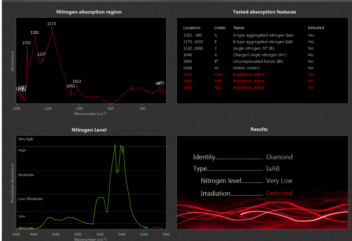
Fig 10. This spectrum belongs to a rare natural low-nitrogen IaAB diamond treated by HPHT, irradiation and annealing in order to change its color to red. The software detected H1a, H1b and H1c– irradiation-related centers and thus warned the operator by displaying a blinking red alert.
