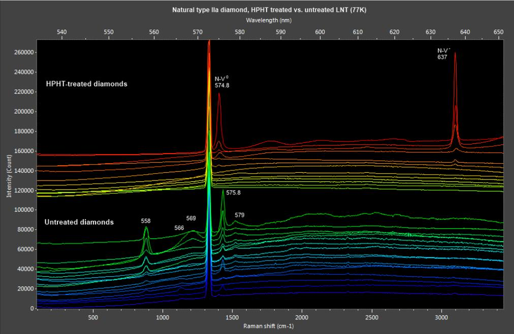
**Detecting HPHT treatment of natural type IIa colorless diamonds**
