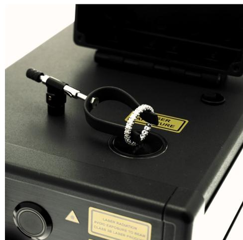
No sample preparation needed. GemmoRaman-532 works on polished, rough and mounted gems. The right image shows the magnetic ring clip accessory in use. Thank to its lightness (4 kg) and very compact footprint (160 x 255 mm), the GemmoRaman-532 is easily transportable. 12 V power supply allows the use even on the field.
