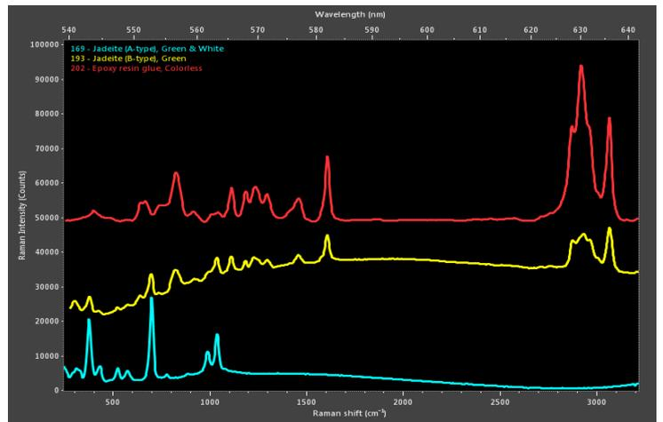
Type A (light blue) and B (yellow) Jadeite Jade compared to epoxy resin (red), Photoluminescence extended range is very useful in order to ID some synthetics and treatments.
