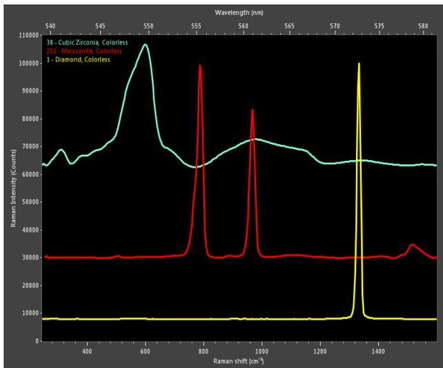
GemmoRaman-532 is an invaluable instrument for fast gem identification. The above image shows a diamond (yellow), a synthetic moissanite (red) and a cubic zirconia (light blue).
